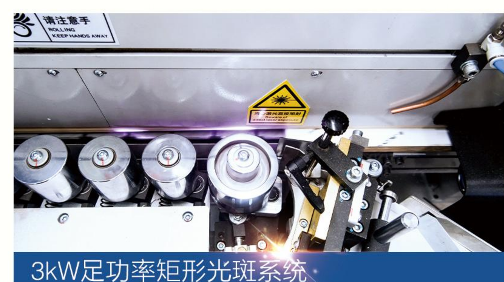
3kW足功率矩形光斑系统 受热均匀，无扫描盲区 Rectangular Spot System The edge is heated evenly
